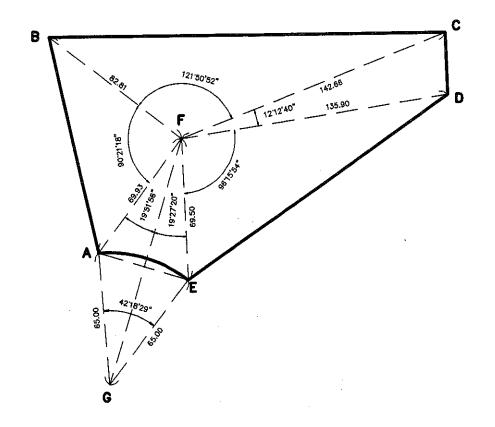
GIVEN: DISTANCE GA = DISTANCE GE = 65.00 ANGLE AGE = 42'18'29" DISTANCE FB = 82.81 DISTANCE FC = 142.66 DISTANCE FA = 69.93 DISTANCE FE = 69.50 ANGLE AFB = 90'21'18" DISTANCE FD = 135.90 ANGLE CFD = 1212'40" ANGLE DFE = 96'15'54" ANGLE BFC = 121'50'52" ANGLE GFE = 19'27'20" ANGLE AFG = 19'51'56"
