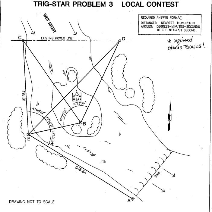
A GROUP OF INVESTORS HAS PLANS TO BUILD A RESORT ON AN ISLAND IN THE WET RIVER. THE ELECTRIC COMPANY WILL SUPPLY POWER TO A TRANSFORMER STATION (Point "B") AT THE RESORT BY CONSTRUCTING A GENERATING PLANT (Point "A") AT THE DAM DOWNSTREAM OF THE RESORT. THE TRANSFORMER STATION WILL NEED TO BE CONNECTED TO AN EXISTING POWER LINE WHICH CROSSES THE RIVER JUST NORTH OF THE ISLAND. USING THE INFORMATION IN THE DIAGRAM THAT WAS OBTAINED BY A SURVEY CREW; FIND THE FOLLOWING DIMENSIONS:
